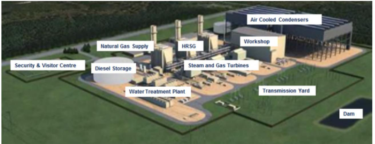
Figure 1 – 3D Illustration of Proposed Installation
